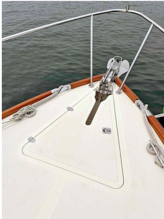
Foredeck Flush Anchor Locker
